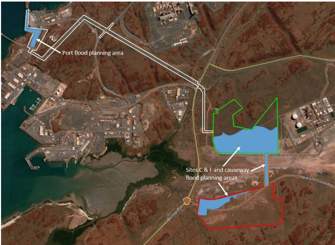
Figure 13-1 Flood Planning Areas at the Port, Site C, Site F and the Causeway (indicative only)
